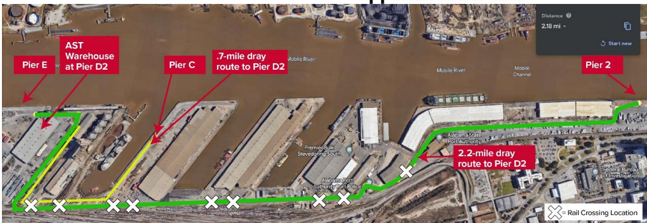
Figure 5: Route Distance for Dray trucks to Pier C and Pier 2 from AST Warehouse at Pier D2
