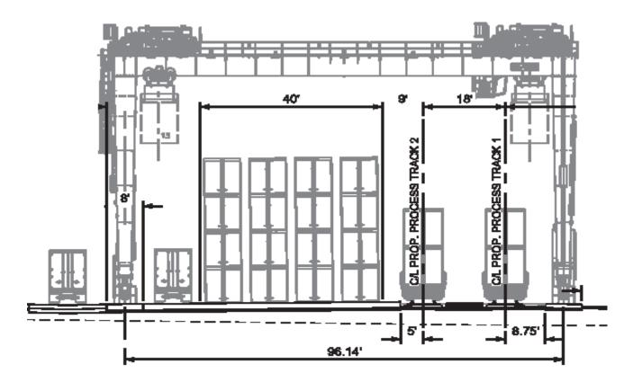
RTG CRANE TYPICAL SECTION
