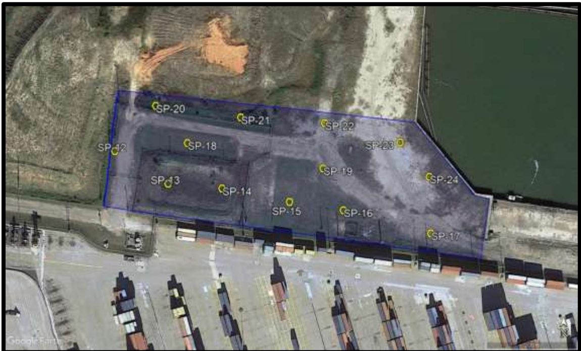
Figure 11 – Initial Surcharge Sites in the Upland Area
