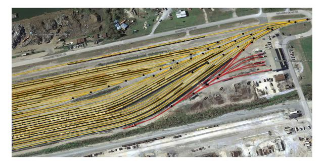
The system will operate by the traincrew entering into the kiosk an ordered list of moves (tracks to switch into) based on their switch list. Once the list is entered the crew begins to switch. The system will line each route in succession as the crew either kicks the cuts or shoves-to-couple. Multiple methods of advancing the routes are provided with the system. Additionally, the system supports switching from anywhere on the ladder and
